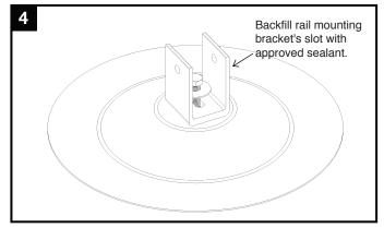
For freeze/thaw locations, a roof manufacturer's approved sealant should be applied around the 3/8" bolt and in the bracket's slot prior to tightening the bolt.
